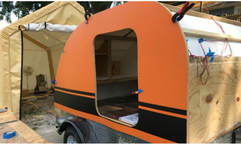
The exterior was skinned with FRP turned to the backside. I used Sherwin William exterior paint and then coated it with Flex Seal rubber coating. The roof is also FRP and sealed with Flex Seal tape. I went this route because I tend to change my mind often, and I knew I would want to change the designs on the sides.
