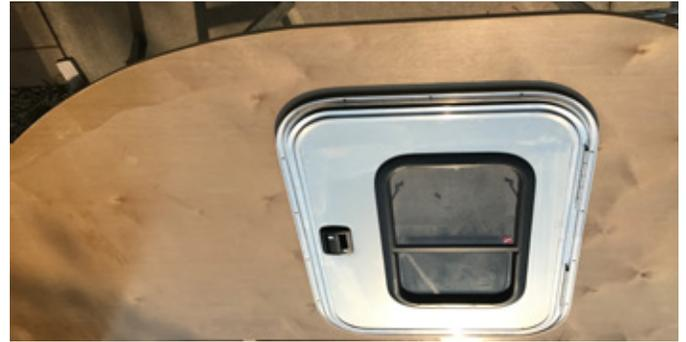
While the plans gave step by step instructions for doors, the awesome guys at Purdy Teardrops (recently purchased by Teardrops NW) sent two silver HEHR prefab doors. I love the built in sliding windows in these doors and the fact they are waterproof. Cutting the holes proved very easy and the install went quick, once I tossed the hand sander and started using the electric palm sander. While, the under-floor storage make the doors sit higher than most teardrops, it has not
