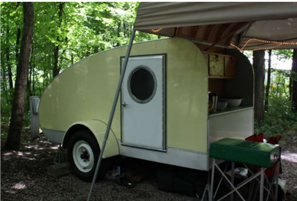
This trailer had a fairly rare front galley style design. The owner took a lot of time with us and explained how it had been built from a variety of reclaimed material and parts. For instance the side panel material is fiberglass laminated plywood cut from the sides of a box truck. The whole family had fun making the most out of their site number with a great Roswell theme. From now on I think I will try to get site 51 when I go camping just so I can do that. Great job everybody. I love it! (Don't worry... I'll give you guys all the credit for the idea.)
